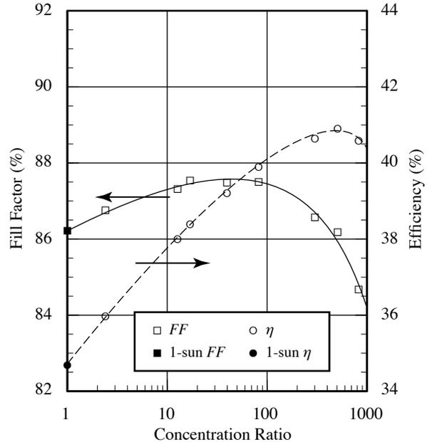
**FIGURE 4.** Fill factor and efficiency versus concentration ratio for the same GaInP/GaAs/GaInAs triple-junction cell shown in Fig. 3 (T-HIPSS data). Subcell photocurrents were correctly adjusted for all three subcells.
