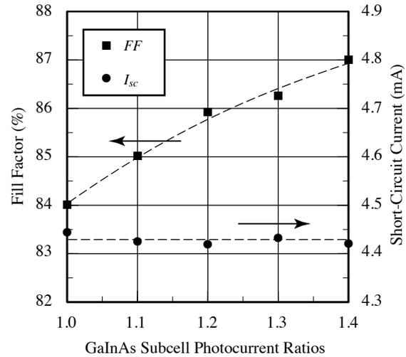
**FIGURE 6.**  $FF$  and  $I_{sc}$  for a GaInP/GaAs/GaInAs triple-junction cell vs GaInAs bottom subcell photocurrent ratios, measured in a 1-sun spectrally adjustable simulator [12].
