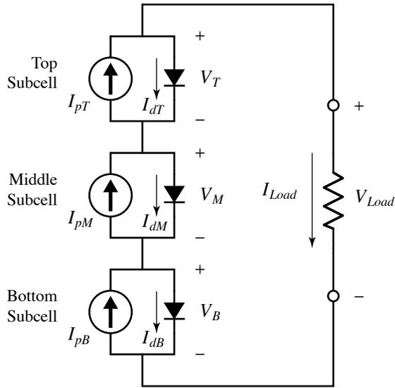
**FIGURE 1.** Simplified equivalent-circuit model of a series-connected triple-junction cell. Parasitic series and shunt resistances are neglected, and the interconnecting tunnel junctions are assumed to be ideal.
