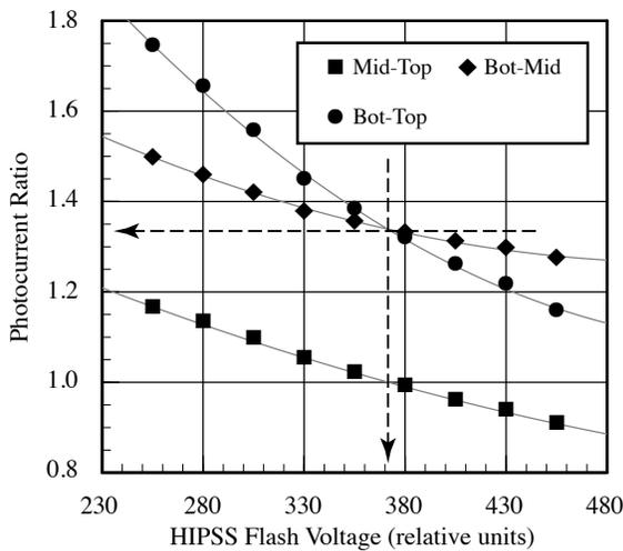
**FIGURE 5.** Subcell photocurrent ratios versus HIPSS flash voltage. The vertical arrow indicates where the middle-top ratio is 1.00 (372), and the horizontal arrow indicates the photocurrent ratios for the bottom subcell (1.34).
