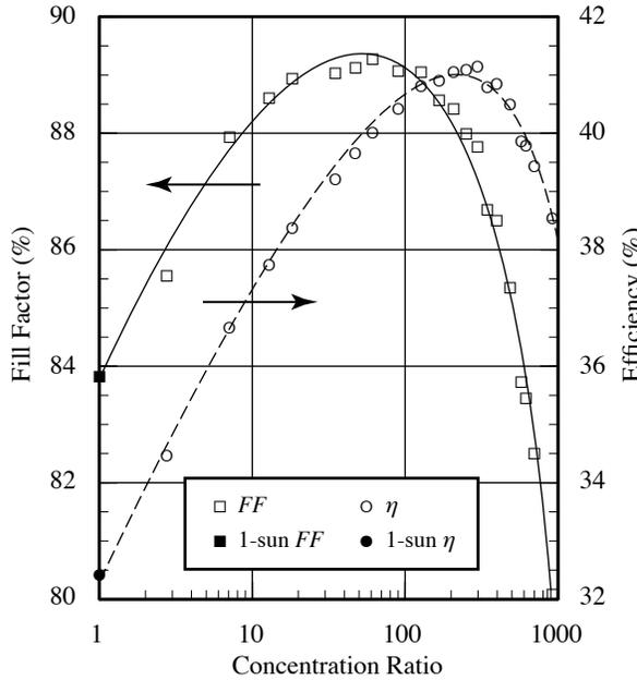
**FIGURE 2.** Fill factor and efficiency versus concentration ratio for a 41%-efficient GaInP/GaAs/Ge triple-junction cell (HIPSS data). The 1× data points were measured separately in a spectrally adjustable continuous simulator; concentration was calculated as the ratio of the HIPSS  $I_{sc}$  to the 1-sun  $I_{sc}$ .
