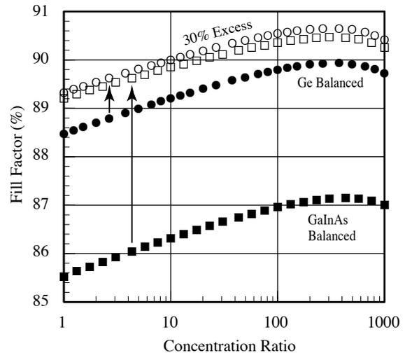
**FIGURE 7.** Modeled  $FF$  versus concentration ratio for two triple-junction cell designs, one with a Ge bottom subcell and the other with a 1-eV GaInAs bottom subcell. The solid points represent the fill factors with balanced photocurrents, while the open points have 30% excess bottom subcell photocurrents.
