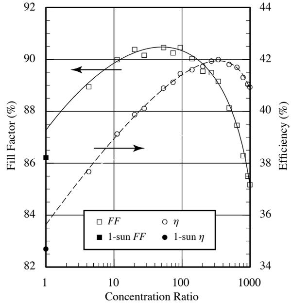
**FIGURE 3.** Fill factor and efficiency versus concentration ratio for a GaInP/GaAs/GaInAs triple-junction cell, measured with the same procedure as that of Fig. 2 (HIPSS data).
