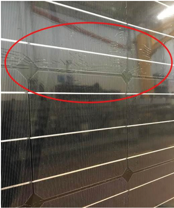
Fig. 5. Detail of wrinkles on the PVB
