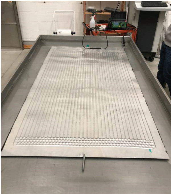
Fig. 7. View of the novel PVT prototype during the wet leakage test
