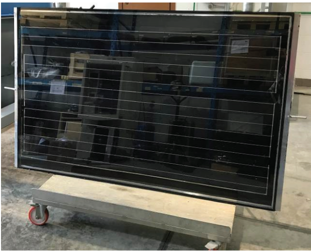
Fig. 3. View of the PVT prototype after the manufacturing process
