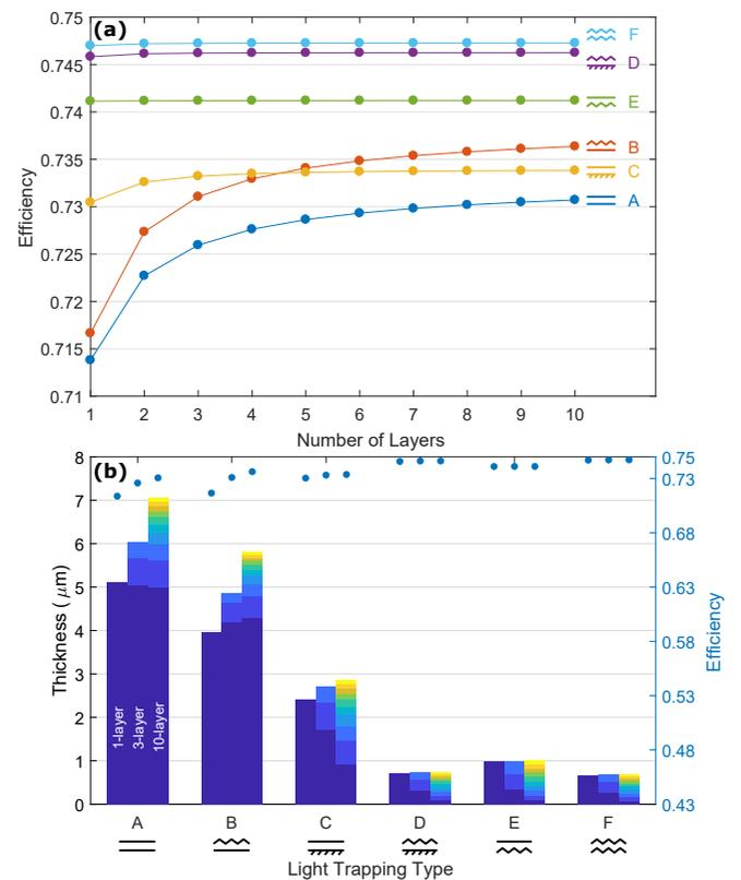
Figure 5. (a) Efficiency, optimized with respect to layer thicknesses, as a function of number of layers for all 6 surface configurations in Table III.  $\eta_{\text{int}} = 0.9$ . Note that A, B have substrates and show the strongest intrinsic efficiency increase with  $m$ . (b) Optimal layer thicknesses of 1-, 3- and 10-layer stack.
