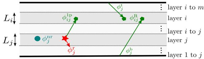
Figure 3. Reabsorption and recombination events in a multi-layer cell.
