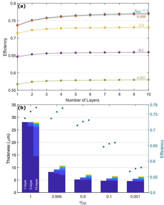
Figure 4. (a) Efficiency, optimized with respect to layer thicknesses, as a function of number of layers with Configuration A in Table II for several values of  $\eta_{\text{int}}$ . (b) Optimal layer thicknesses of 1-, 3- and 10-layer cells (left axis, bars) and the associated efficiencies (right axis, points). Each color shows a single layer.
