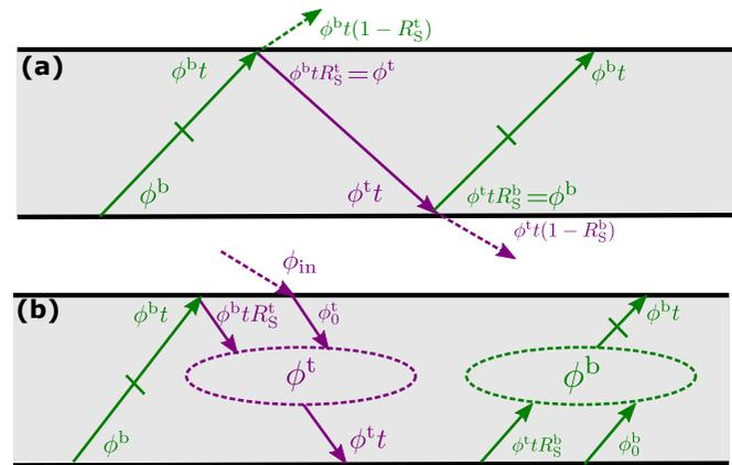
Figure 2. Self-consistency relation between top and bottom inward photon fluxes,  $\phi^t(\theta, E)$ , and  $\phi^b(\theta, E)$ , (a) without source terms and (b) with source terms  $\phi_0^t(\theta, E)$  and  $\phi_0^b(\theta, E)$ . Figure shows specular top and bottom surfaces. In the case where the source is from external radiation  $\phi_{\text{in}}$ ,  $\phi_0^t = \phi_{\text{in}}(1 - R_{\text{ext}})$ .
