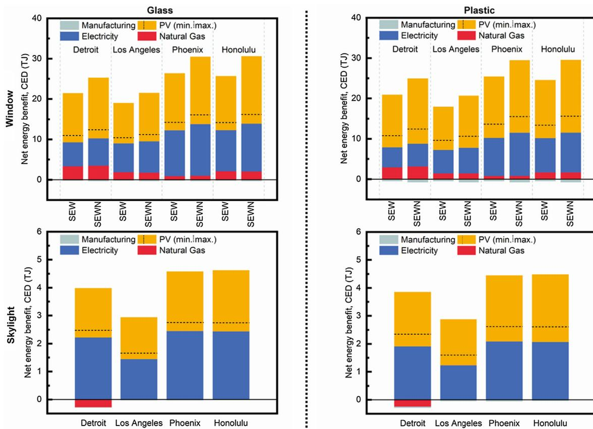
Fig. 6. Net cumulative energy benefit for glass and plastic TPV for window and skylight applications for all four locations. The photovoltaics electricity generation was based on the current (min:  $\eta = 3\%$ ,  $T_{50} = 7$  yrs) and future (max:  $\eta = 10\%$   $T_{50} = 25$  yrs) technologies.
