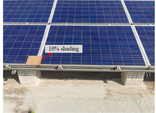
Fig. 4. Photograph of the experimental scene under one cell 10% shading.
