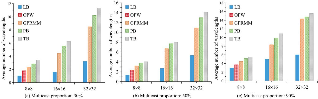
Fig. 7. Average number of wavelengths of GPRMM, TB, PB in  $8 \times 8$ ,  $16 \times 16$ ,  $32 \times 32$  mesh ONoC under different multicast proportions.
