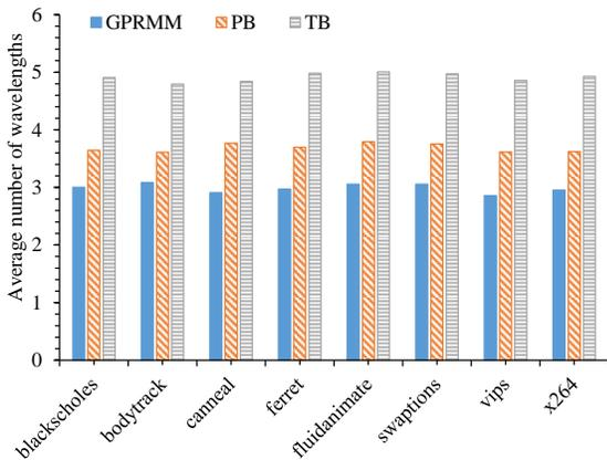
Fig. 8. Average number of wavelengths in different applications of trace-based simulations.
