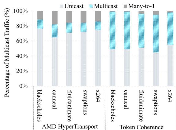
Fig. 1. Traffic percentage for a set of standard PARSEC benchmark applications for Token Coherence and HyperTransport in a 64-core system [11].
