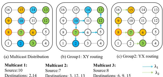
Fig. 3. Illustration of the proposed multiple multicasts routing scheme.
