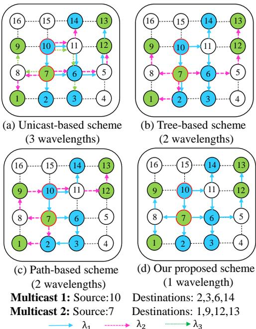
Fig. 2. Routing examples for multiple multicasts in a 4x4 ONoC.
