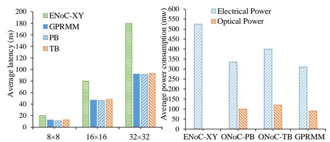
Fig. 9. Performance comparison for different routing schemes, (a) average latency under different network sizes; (b) power consumption under  $8 \times 8$  mesh network.
