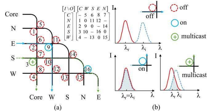
Fig. 6. The principle of multicast-enabled optical router, (a) the router architecture for a single wavelength; (b) different switch status by tuning the resonant wavelength of MR.
