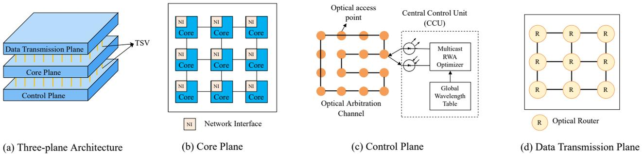
Fig. 5. A three-plane ONoC architecture for implementing GPRMM.
